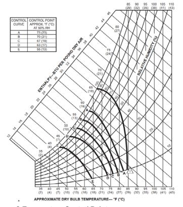
Figure 1. Enthalpy Sensor & Temperature Control Points
