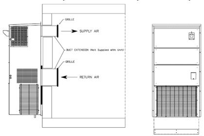
Figure 4. Mounting Unit on a Wall
