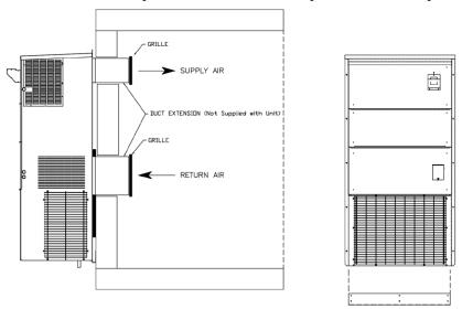
Figure 4. Mounting Unit on a Wall
