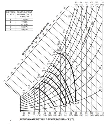
Figure 1. Enthalpy Sensor & Temperature Control Points
