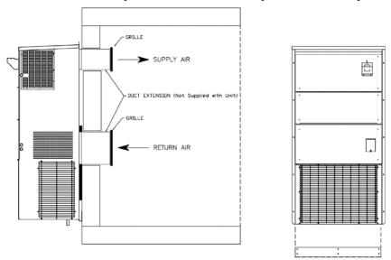
Figure 4. Mounting Unit on a Wall
