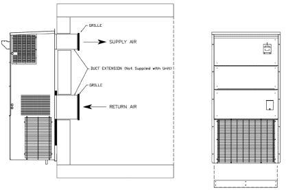
Figure 4. Mounting Unit on a Wall
