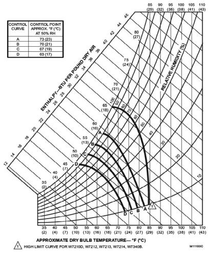
Figure 2 - Enthalpy Sensor Temperature Control Points
