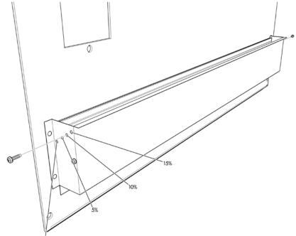
Figure 3 - Fresh Air Hood Damper Adjustment
