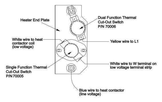
Figure 10 - Typical Configuration for Single Element Heater
