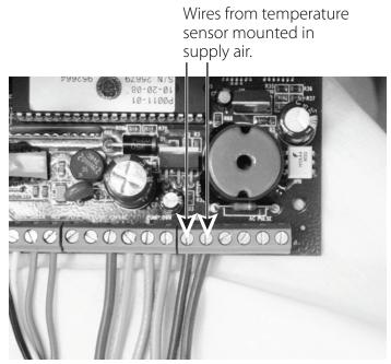
Figure 6 - Temperature Sensor Wires
