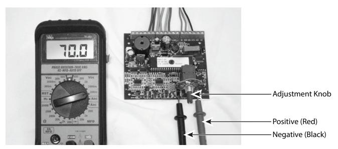
Figure 7 - Desired Temperature Set Point
