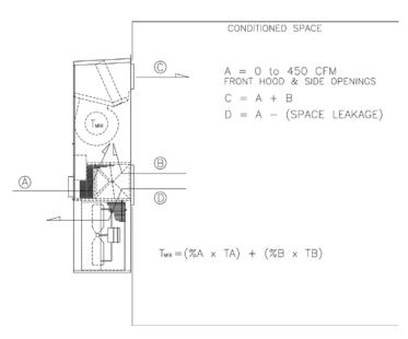
Figure 9 - Damper Air Path
