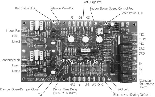
Figure 1 - PC Control Board
