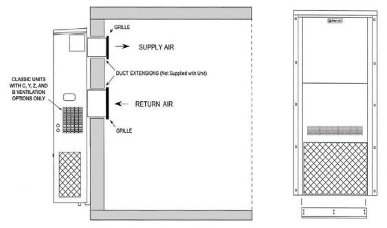
For units with electric heat, a 1" clearance around the duct extensions is required. The duct extensions must be made of galvanized steel with a minimum thickness of .019" as per the NFPA standards 90A & 90B.
